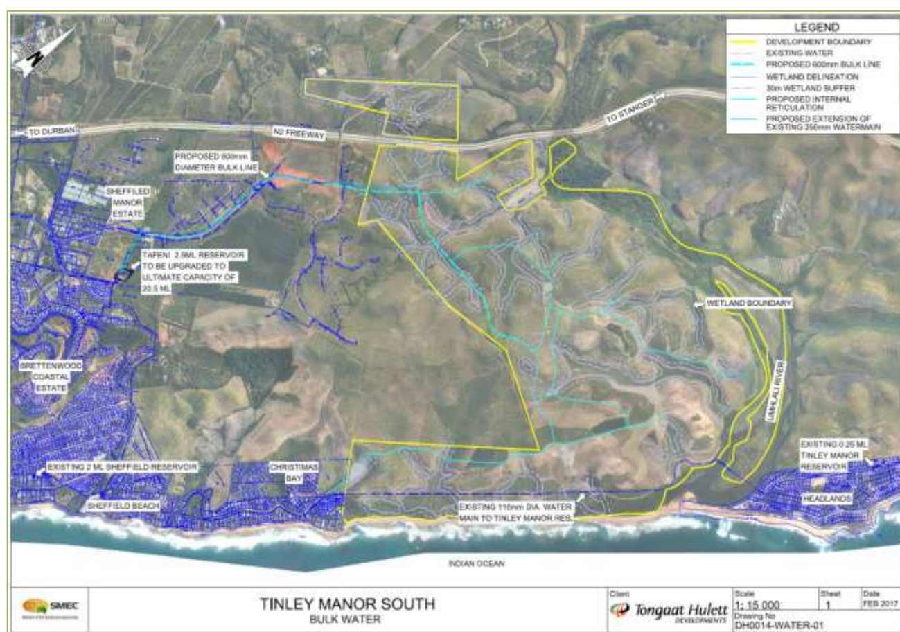
Figure 3-11: Proposed bulk water network
